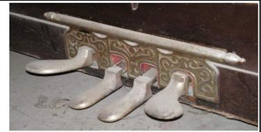
The home or apartment version (bottom right) used the fourth pedal to lower a wooden bar down in front of the hammers that would completely dampen the sound. This allowed the player to play without disturbing others within the home or apartment or the neighbours.
